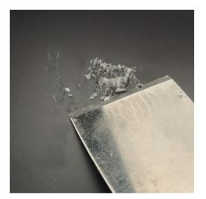
● If there has some glue hard to be clean off by scraper, please put the plate back and set the bed temperature to be 230 °C and wait for about 30 minutes. Then try with scraper again.
